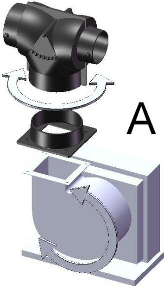
Configure our AirDividers by first choosing one of two inlet supply types (Adapter on left or Hose on right). Both begin with a blower adapter secured to your unit. If you want to mount our AirDivider directly onto the blower specify "A". The draft angle on our blower adapters is a perfect fit for our A-style AirDividers. Rotate the AirDivider as necessary and secure. If you will be connecting to the blower with hose duct specify "H" and secure duct on all fittings.
