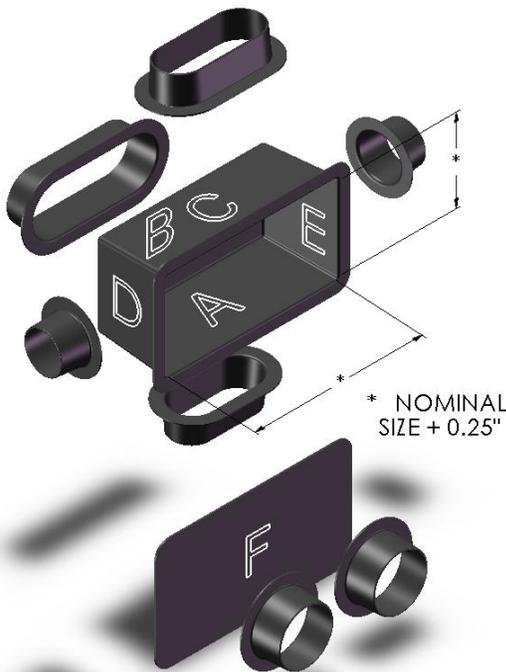
Our standard transition boxes are constructed of black ABS with a haircel finish. They are all slightly more than 5" deep and at the opening they are 1/4" larger than the nominal size. The flange corners and all edges are rounded to avoid sharp points.
