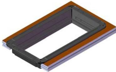
Installed into the sides of the grille are stainless steel spring catches. They secure the blade/track assembly inside the grille frame but their primary purpose is more functional. They hold the grille into what we call a mounting frame. This mounting frame (MF) is constructed of four injection-molded corners and four pieces of extruded sides glued together. It is mounted from the finished side of the wall and then the grille is “snapped” into it. Grille removal is just as easy.
